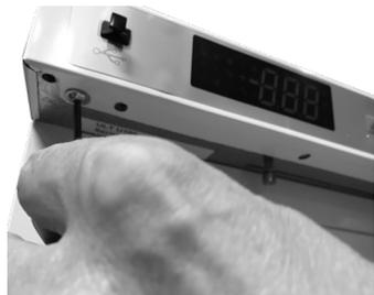
4. Remove screws underneath the top-panel (use 3 mm allen key)
