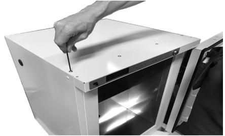
2. Loosen and remove visible top screws (use 3 mm allen key + Torx 20 tool)
