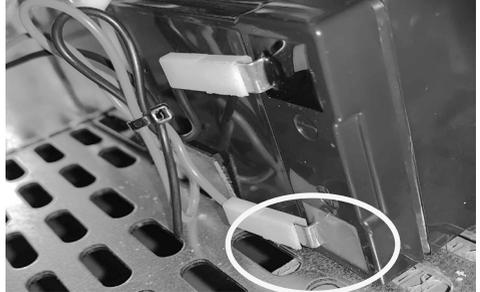
Remove motorcover and attach red wire with receptacle to “+” pole of battery. This will switch on the battery backup system.
