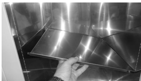
Lift up to release all hooks and pull the shelf to one side. Then tilt the shelf upwards in the free side and lift it out
