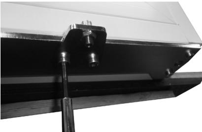
29. Remount bottom handle lockpin plate in the opposite side by tightening the two screws again (use 4 mm allen key)
